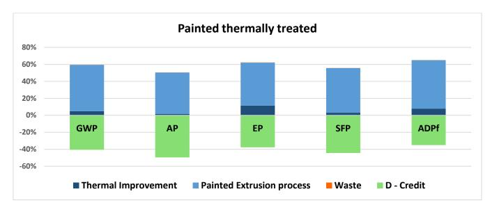
Figure 10: Painted thermally treated extrusion LCIA results by manufacturing stages
