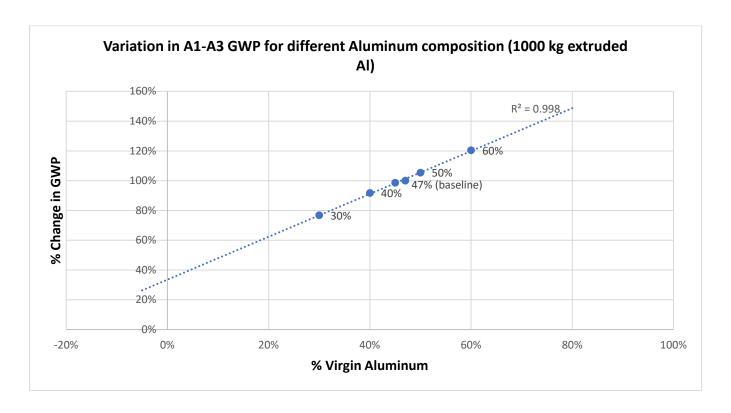
Figure 11: Sensitivity analysis - impact of primary ingot and recycled content on mill-finished Aluminum extrusions
