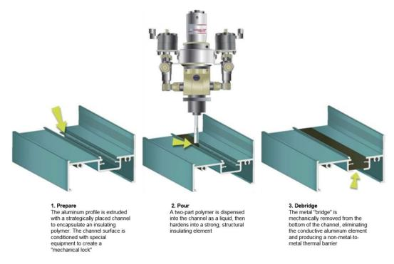
Figure 2. Pour and debridge process
