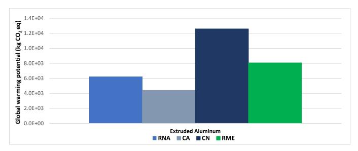
Figure 12 : Effect of source of primary aluminum on cradle-to-gate carbon footprint (RNA: North America, CA: Canada, CN: China, RME: Middle East)
