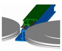
**3. Crimping**Three sets of wheels rotate the extrusion onto the Strip and mechanically lock the components together. Over 1300 pounds of pressure is applied in stages, and the resulting aluminum/Strip assembly will then act as a load-bearing composite. Shear testing is typically conducted periodically to verify that the process has produced an assembly that will perform structurally as
